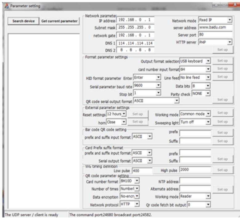
2. Use mini USB data cable connect the QR code reader to PC, fill-in light on, buzzer rings, QR code reader start done, then use the internet cable connect the QR code Reader to PC.
